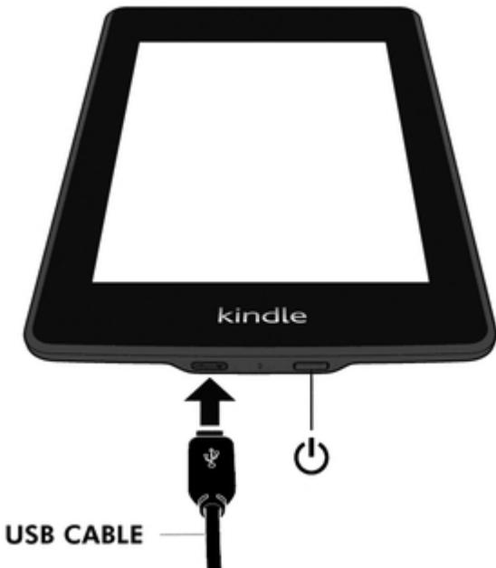
**Power button:** To turn your Kindle on, press the Power button located on the bottom edge. If you need to turn off your Kindle screen, press and hold the Power button for 7 seconds until the Power dialog box displays and then tap Screen Off.
